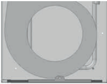
How to remove the filter from A/P units. Turn the filter holder as shown. Remove the filter.
